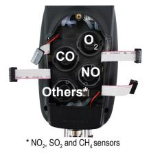
When a sensor has been replaced, it is possible to check the proper functioning of this new sensor by going in the "Information" menu of the analyser. It is normal that a sensor that has just been installed gives the following message: "Current Error", it is necessary to wait a few time to stabilise the polarisation of the sensor.
