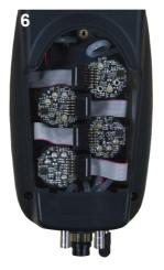
Connection of the sensor ribbon cable
