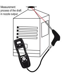
Put the probe of the KIGAZ 310 in the draft hood, going through the side openings of the boiler
