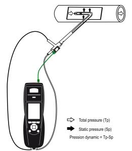
The Pitot tube must be introduced perpendicularly, in the middle into the duct and parallel to the flow.
