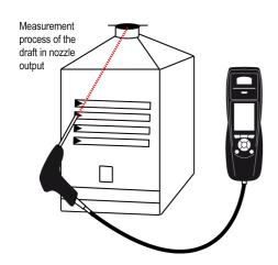
Put the probe of the KIGAZ 310 in the draft hood, going through the front face of the boiler
