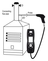
Put the probe of the KIGAZ 310 in the nozzle output, from the beginning of the connecting flue
